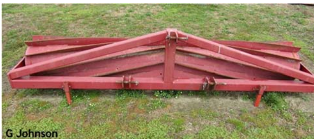
Chevron bladed roller crimper for rolling cover crop prior to transplanting
